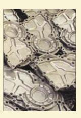
What is die-casting? Most people probably have little more than a vague idea of this fundamental industrial process but it is vital to a huge variety of manufacturing operations where metals have to be forced into a metallic mould so as to produce a part of the right shape and dimensions. That is die-casting.
