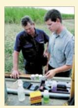
Now the CRC for Sustainable Sugar Production (CRC Sugar) has produced a relatively simple kit that can be used to test for sodicity in the field. So long as farmers have a basic understanding of soils they can soon do the testing themselves, once they have gone through a short training session. The kit contains materials and instructions for three different field tests.
